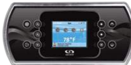
in.k800 main keypad Color LCD display, 10 keys
