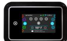
in.k1000 main keypad Color LCD capacitive touchscreen display
